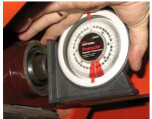
**NOTE:** EFI makes it possible to set more radical angles for your powertrain because it does not rely on level float bowls like a carburetor. However, the driveline angles at your u-joints are important for a smooth, steady driveshaft rotation. Even with EFI you should try to maintain the  $-3^\circ$  powertrain angle.
